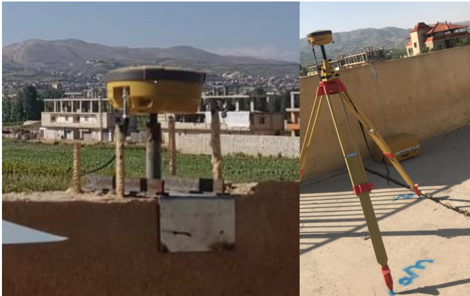
Fixed Tribrach with antenna oriented North installed on unknown Point B
