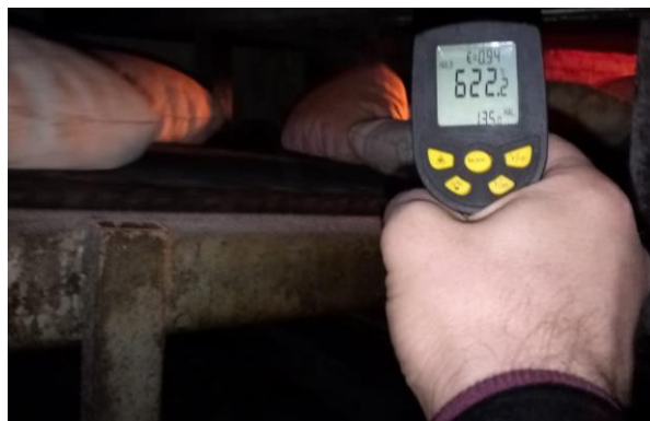
Figure (1) shows the method of measuring the temperature inside the baking room
